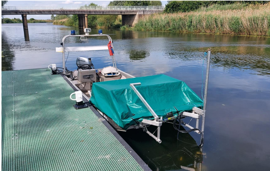
Image 4: The Reeve showing twin bow acoustic mounts
